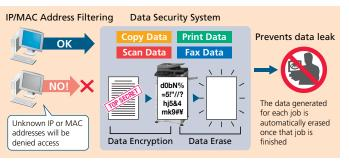
Attempted access from an unknown IP or MAC address will be denied, preventing unauthorised use. The MX-2314N also supports the **IEEE 802.1X** standard for port-based network access control, which blocks all access from unauthorised devices.
