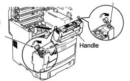
(5) Press and secure blue lock control lever on the left and right of the fuser unit.
