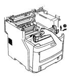
(4) Remove the toner cartridge carefully from the machine.
