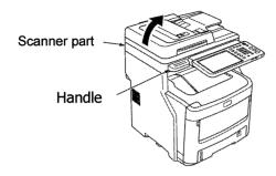
Press the top cover open button to open the top cover.
