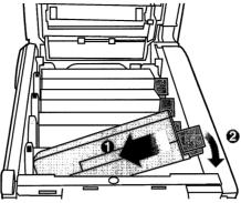
**12.** Pressing gently down on the cartridge to ensure that it is firmly seated, push the coloured lever (1) towards the rear of the MFP. This will lock the cartridge into place and release toner into the image drum unit.
