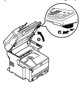
2. Press the cover release (a) and open the top cover (b) fully.
