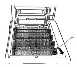
**5.** Lift the right-hand end of the cartridge and then draw the cartridge to the right to release the left-hand end as shown, and withdraw the toner cartridge out of the MFP.
