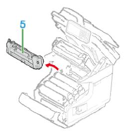
7. Hold the handle and place the new fuser unit into the machine.
