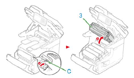
5. Pull forward the left locking lever (4) of the fuser unit to unlock.
