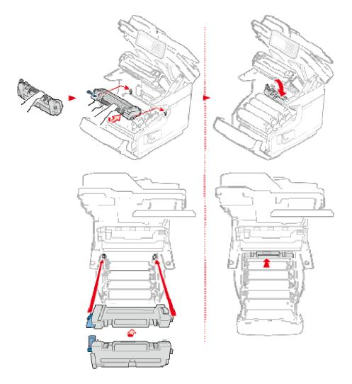
8. Push back the left locking lever (4) of the fuser unit to lock.
